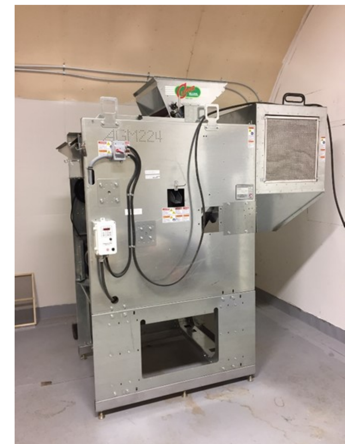
Figure 5. ACM 224 Clipper with screens for cleaning grass and legume seed samples.
