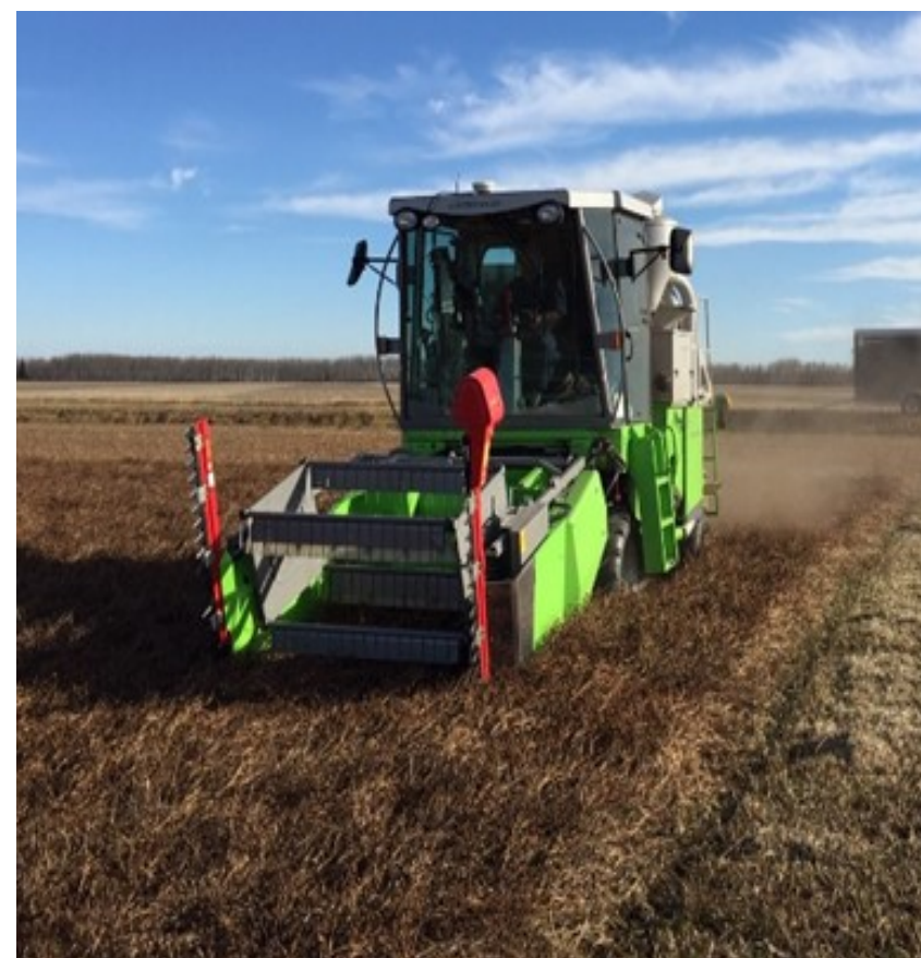
Figure 1. Straight cutting alsike clover using Wintersteiger combine equipped with sidecutters.
