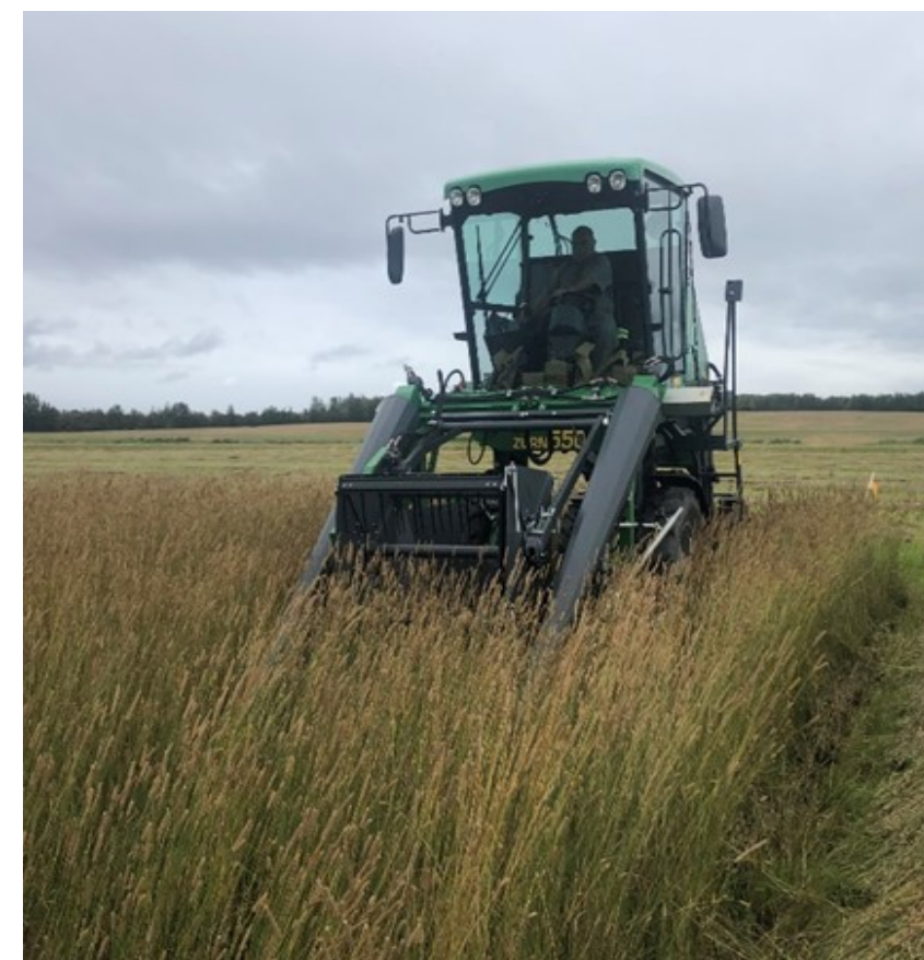
Figure 3. Swathing growth regulator trial on timothy using Zurn 550 Multifunctional Tool Carrier.
