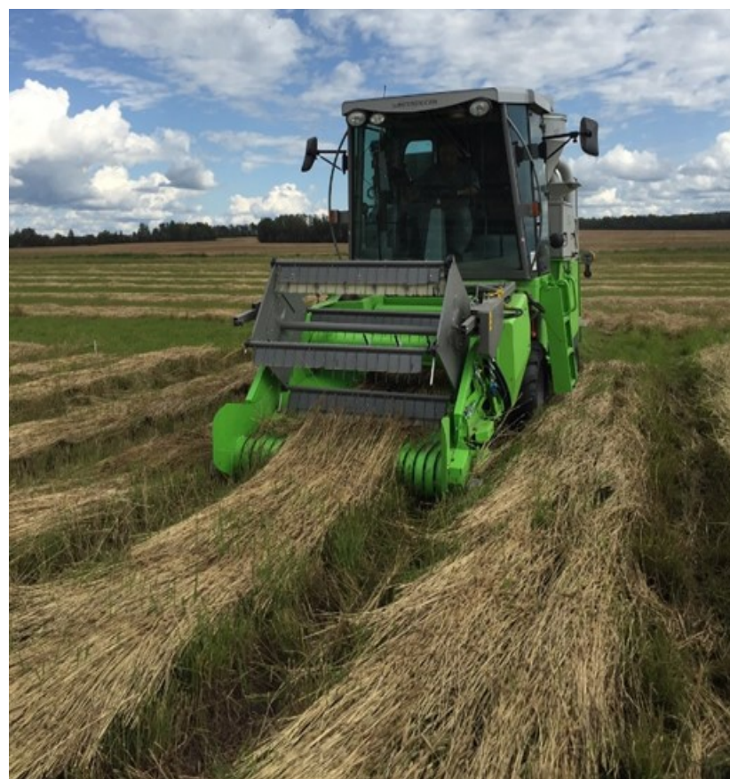
Figure 4. Combining timothy swaths with new pickup header on Wintersteiger combine.
