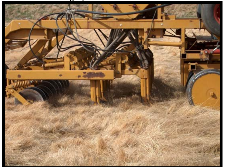
Above and below: A photo during seeding operations on May 10 th . The fine job that the Haybuster 8000 does of seeding into heavy fescue sod can be clearly seen. The coulters do an excellent job of cutting the sod ahead of each shank resulting in a very smooth field after seeding operations.
