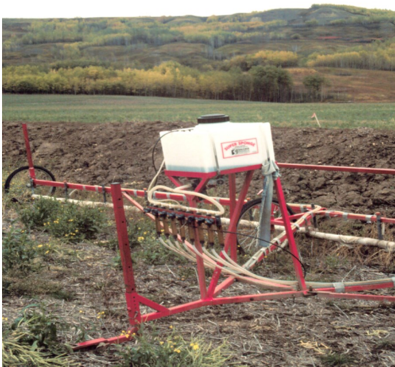
Smucker wick applicator for wiping glyphosate to eliminate quack grass in grass seed fields.
