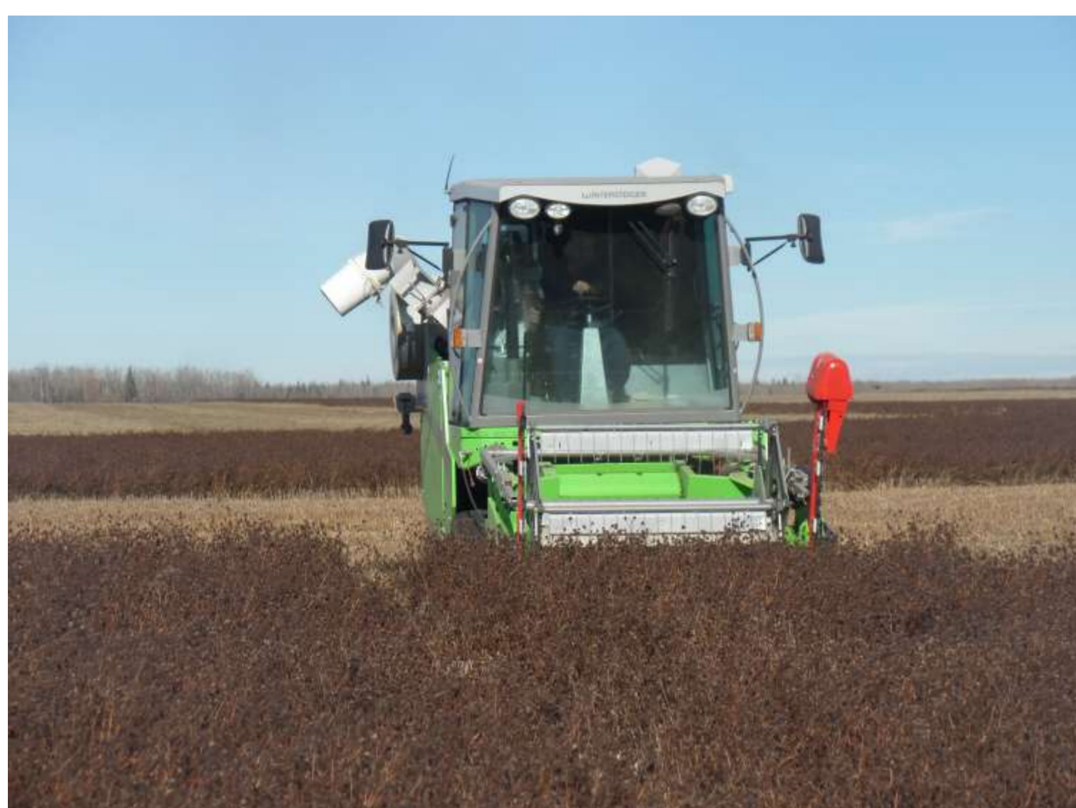
Figure 3. Harvesting red clover seed with SARDA small plot combine.
