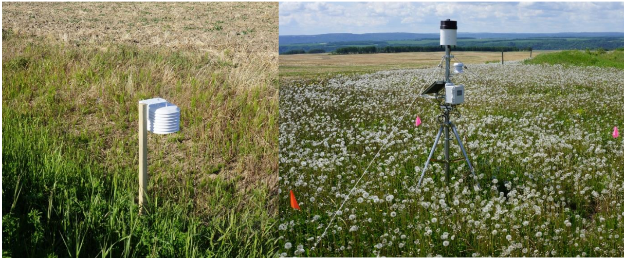
Left- Manual shuttle weather station; data collected ~twice a year for long term use. Right- Internet accessible data transferred automatically via cell network; annual subscription fee, but reliable and can be used weekly for forecasting.
