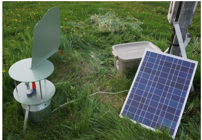
Phytoshield AAFC project. A spore sampler draws in air continuously which is filtered into a collection vial. All of the contents are collected weekly then sent to the researchers; they have started using the data to build PCR diagnostics (tools for using DNA to identify organisms) for cereal pathogens across western Canada. This site is maintained in Fort St. John BC and stewardship has been transferred to the BC Grain Producers association.
